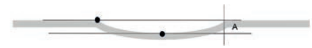
The deformation value is the height difference A between the two points shown
