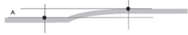
Deformation value is the height difference A between the two points shown.
