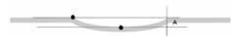
The deformation value is the height difference A between the two points shown
